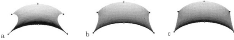
Fig. 6. Combination of SSDM and FDM for different values of coefficients a) q_{sj} = 1 and q_{ij} = 6 b) q_{sj} = 1 and q_{ij} = 25 c) q_{sj} = 1 and q_{ij} = 100
